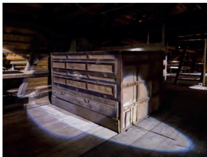
Hop drying kiln with two levels of folding blinds in the exhibition Sušička se dvěma patry sklopných žaluzií v expozici
